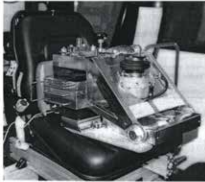
Fig. 2. Testing of a motor vehicle seat with the use of a dummy [4]
